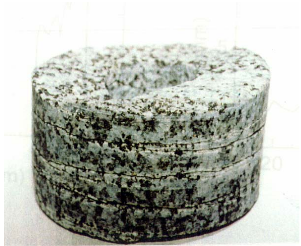
Core discing which was observed at Kamaishi Mine
