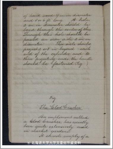
of hard wood 9 in. in diameter and 5 or 6 ft. long. A hole, 2 in. in diameter should be bored through the center of this. Through this hole should be passed an iron axle 2 in. in diameter. This axle should project 2 or 3 in. beyond each end of the cylinder, and to these projecting ends, the handle should be fastened. (Fig.)
