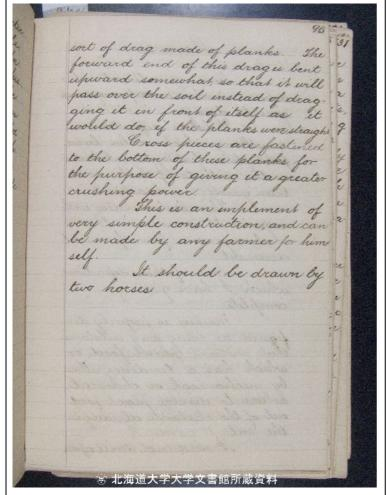
sort of drag made of planks. The forward end of this drag is bent upward somewhat, so that it will pass over the soil instead of dragging it in front of itself as it would do, if the planks were straight.
